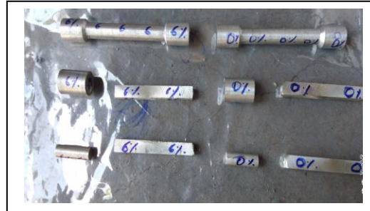
Fig.2 Tensile, Compression, Impact and Wear test specimens
